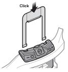
2. Pull the release tool until the main unit comes off the helmet.
